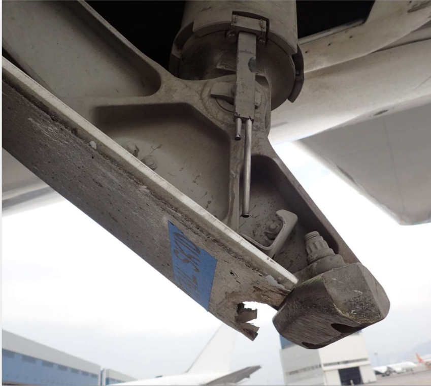
Photo 2: Tail Skid Damage
