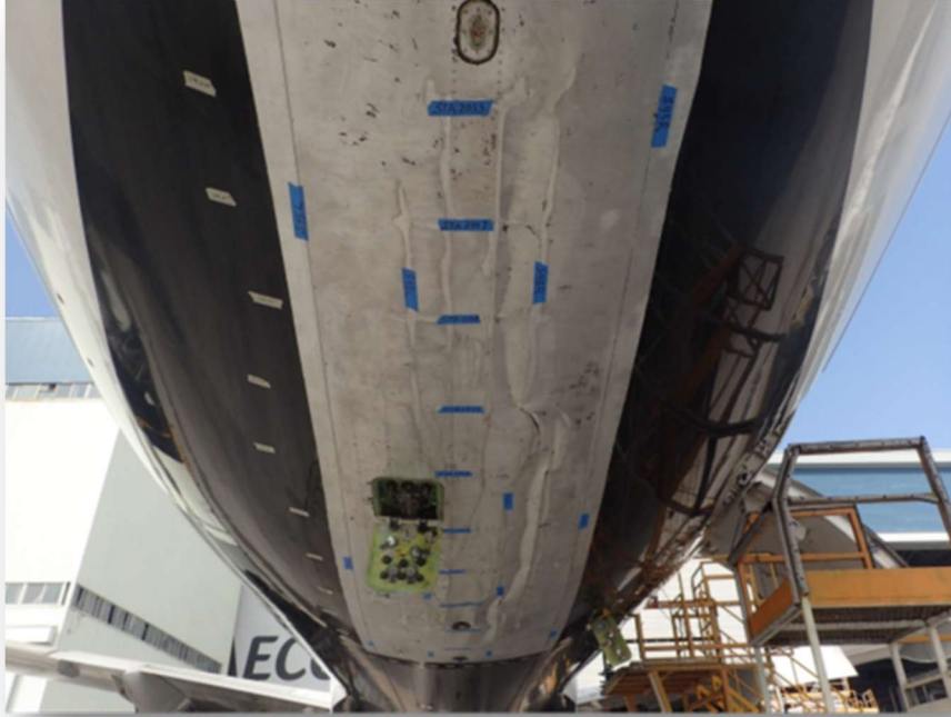
Photo 4: Lower Aft Fuselage Damage (2)
