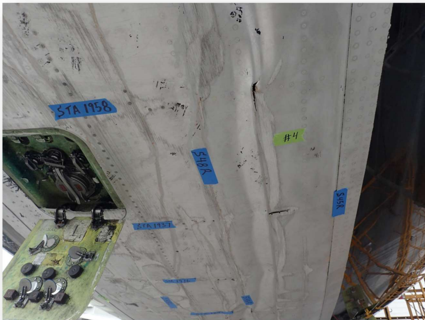
Photo 3: Lower Aft Fuselage Damage (1)
